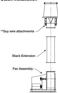
If fan requires a stack or stack extension, install on fan before installing nozzle and windband. Place gasketing between any sections, blower housing and initial stack. Use lifting lugs to position each piece into place. Attach stack or stack extension to blower housing using 316 stainless steel bolts (provided) through flanges aligning bolt patterns. Use antiseize gel (provided) to prevent galling/welding of all stainless steel fasteners.
